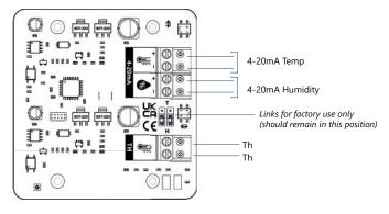
Typical connection diagram with external power supply
