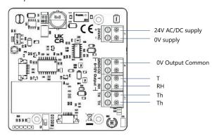
Typical connection diagram for with power supply from BMS controller
