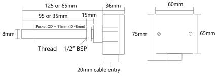
Sensor is supplied with cable entry gland fitted
