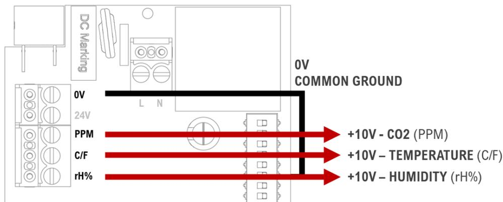
In normal operation, output levels are proportional to the gas level as shown below.
