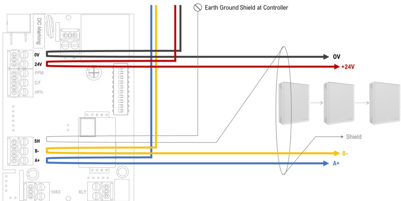
Daisy chain wires running to additional RS sensors – 127 sensors max per cable run. First and last device in bus requires a termination resistor. Use EOL switch to terminate RS sensor. Recommended 3-core, 2 twisted pair + ground, shielded cable with 120  $\Omega$  characteristic impedance.
