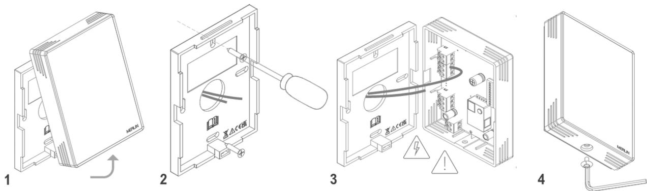
1. **Remove the front cover** by removing the screw underneath the housing using an M3 socket wrench.
